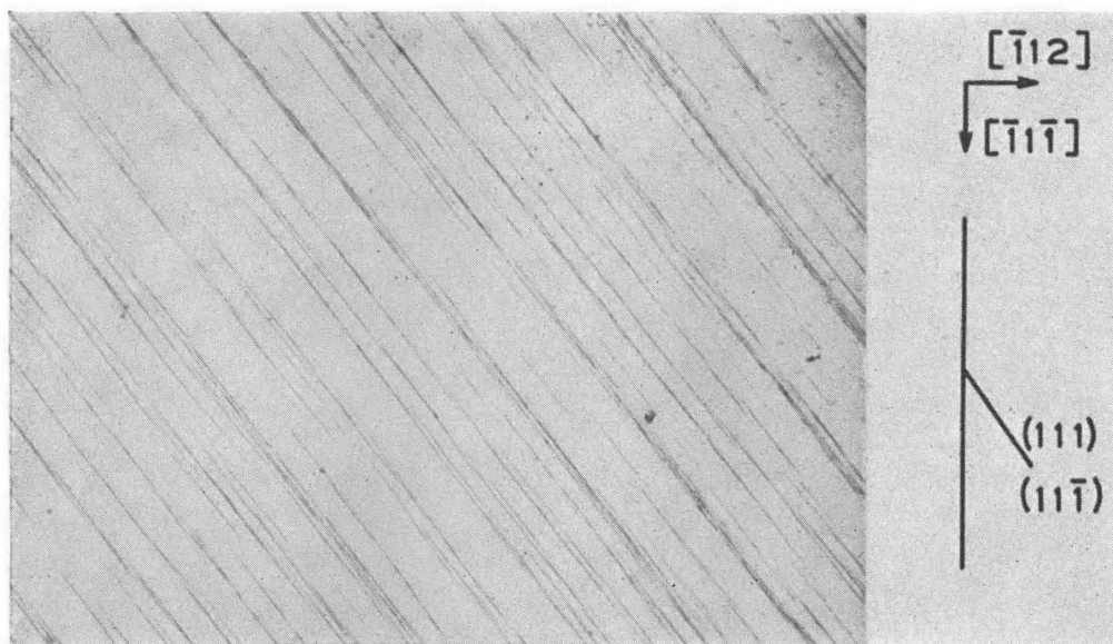
FIG. 8. Top surface of (110)[112] Permalloy crystal after 50.5% thickness reduction, electropolished, and then further deformed lightly. No constraint on \epsilon_{y_2} . Slip plane traces consistent with predicted -a_2 , (111)[101], and b_2 , (111)[011] slips. \times 140
